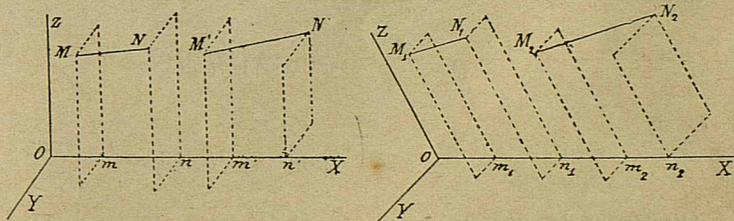
$$m n = o n - o m \left\{ \begin{array}{l} o n = \text{abscisa de } N = x' \\ o m = \text{» } M = x \end{array} \right. \text{Proyección de } M N = m n = x' - x$$
