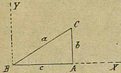
$$\left. \begin{array}{l} \text{sen } B = \frac{b}{a} \gg b = a \text{ sen } B \\ \text{cos } B = \frac{c}{a} \gg c = a \text{ cos } B \\ \text{tg } B = \frac{b}{c} \gg b = c \text{ tg } B \\ \text{cot } B = \frac{c}{b} \gg c = b \text{ cot } B \end{array} \right\} \text{ y substituyendo } B = 90^\circ - C \text{ se tendrán las restantes.}$$
